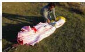
**Step 5** Strap the Folding Pillow below the LE - at the point of the first fold. The pillow reduces the angle of the fold and helps preserve the plastics. Next fold the TE around the LE being careful to not fold with tight angles
